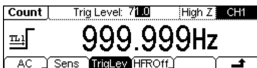
Figure 2-65 To set the trig level
