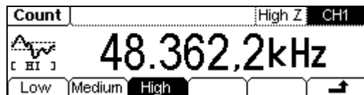
Figure 2-64 To set the sensitivity
