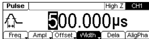
Figure 2-13 Pulse Signal Parameter Setting Interface
