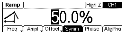
Figure 2-10 Ramp Signal Parameter Setting Interface
