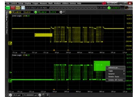
Identify signal integrity issues with InfiniiScan Zone – Qualify triggering.
